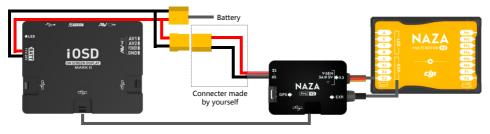
Fig.2 Connection between iOSD and NAZA-M V2
