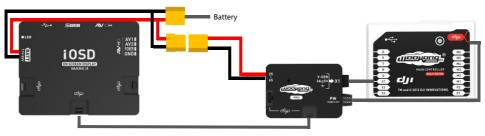
Fig.3 Connection between iOSD and WKM
